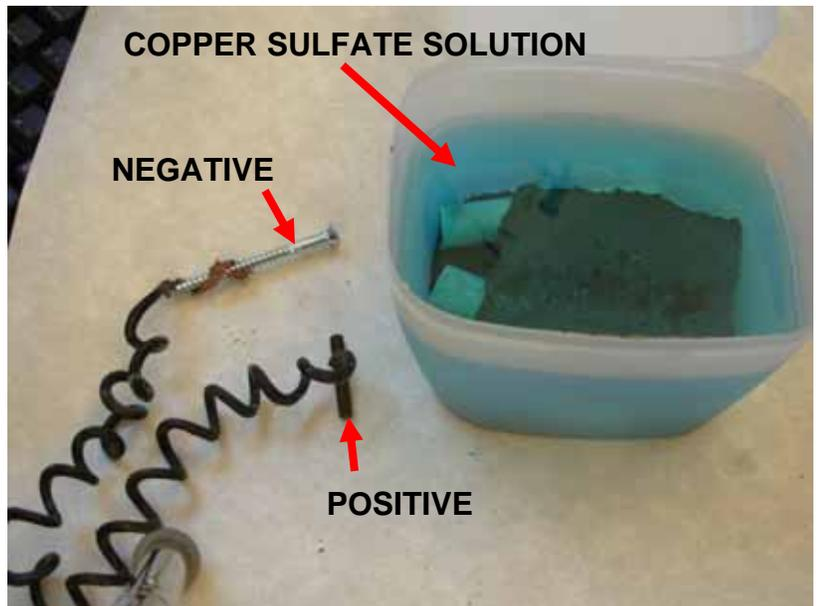
I wrap the wires around a rod so that the negative terminal has a large exposed surface area. Put the negative terminal in the bottom of the bath.
