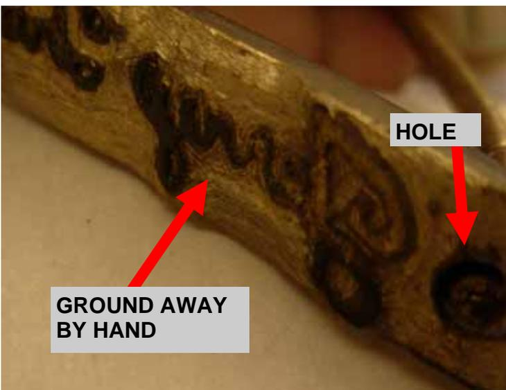
Drill one hole at each end of the design. Size the hole so that 1/8 brass rod will fit easily. If the fit is too close, then you may have trouble getting braze to flow in between the rod and the hole.
