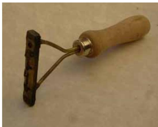
Loosely fit the rods in the brand extending away from the design and braze them to the brand (use acetylene or MAP gas). I use brazing because it is more durable. Because you're not going to heat the brand to the melting point of solder when you use it, you may be able to get away with plumbing solder to join the rods to the brand.
