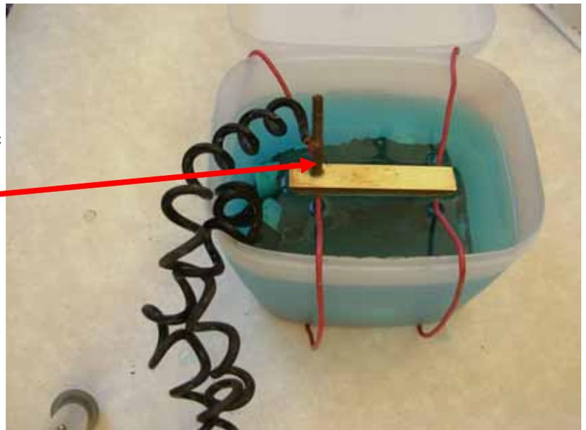
Attach the positive bath lead to the positive lead on a battery charger. Attach the negative bath lead to the negative lead on the charger, and turn the charger on. Make sure that the charger is working properly and isn't overloading.
