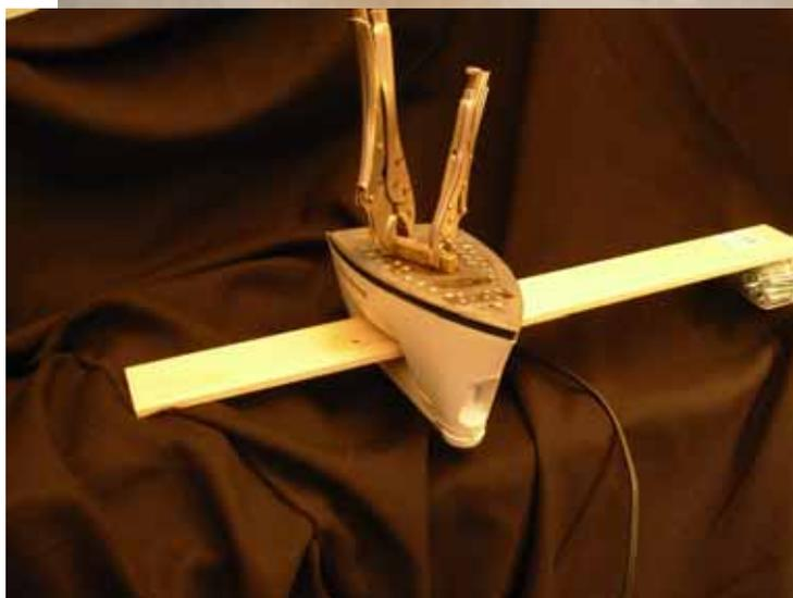
Carefully take the brass off the iron and release the vice grips. Drop the brass into soapy water. The two pieces of brass will stick together. Soak the brass for about 15 minutes to release the two pieces of brass from each other. Don't pry the two pieces apart, since that can ruin the resist. If the two pieces don't readily come apart, slip an exacto blade between the two pieces and rock it very gently to separate the pieces slightly, then put them back into the soapy water to soak.
