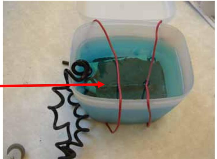
Suspend the brass bar at the top of the bath, making sure that the wires that suspend the bar don't touch the design. I attach the positive lead to a short piece of rod or a small bolt and rest it on top of the brass bar to complete the circuit in a way that can easily be disconnected.
