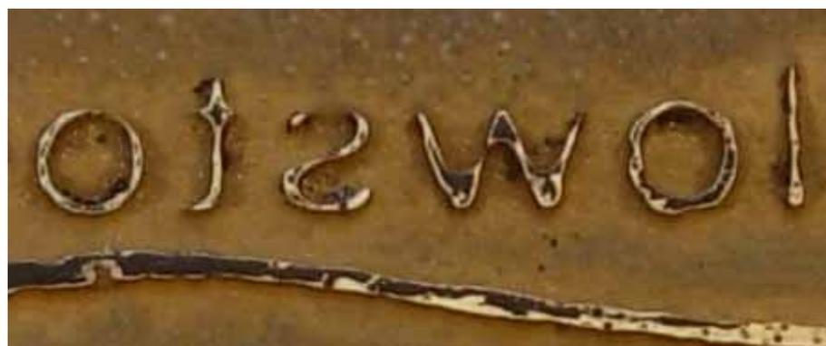
Use a Dremel drill to grind away the brass away from the raised design. If the design has fine spaces between parts of the raised brand, use an Exacto knife to gouge out the brass. You want the design to be the highest part of the brand, and the surface of the brand should slope down around the design.
